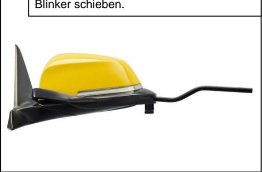
The image shows the yellow mirror housing with the black bracket now fully attached to its back. The bracket is positioned under the blinker mechanism.
