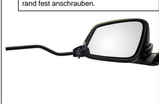
The image shows the mirror housing with the bracket attached. A black screw is being used to tighten a clamp on the bracket, securing it to the mirror housing.
